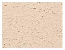
Structure of a gypsum cardboard panel prepared with YELLOW primer
