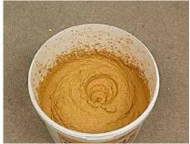
Mix well again after 30 minutes, the picture shows the consistency of ready-to-use mortar
